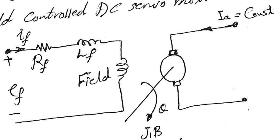
The electric circuit is modelled as,
