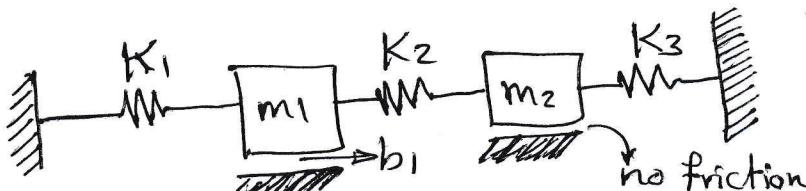
Q4 write the equations of motion of figure below.
