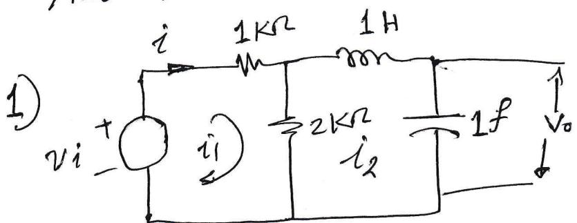
$$\textcircled{a} \frac{v_o(s)}{v_i(s)} \quad \textcircled{b} \frac{v_o(s)}{i(s)} \quad \textcircled{c} \frac{i_2(s)}{i(s)} \quad \textcircled{d} \frac{i(s)}{v_i(s)}$$
