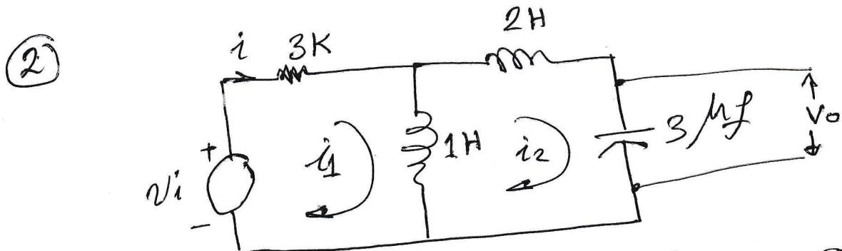
$$\textcircled{a} \frac{v_o(s)}{v_i(s)} \quad \textcircled{b} \frac{v_o}{i(s)} \quad \textcircled{c} \frac{i_2(s)}{i(s)} \quad \textcircled{d} \frac{i(s)}{v_i(s)}$$
